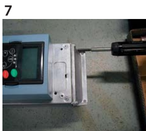
7 Fix the top flange to its place.
