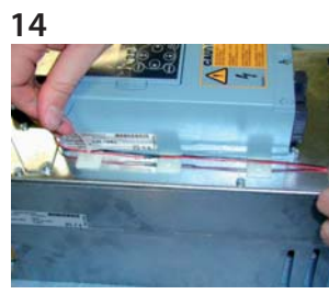
14 Attach the adhesive-backed mount (7) as shown in the picture and use the ties (#5) to fix the cables on the power unit.
