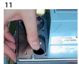
11 Seal the air inlets with the rubber sealings (#4). Leave the opening uncovered.
