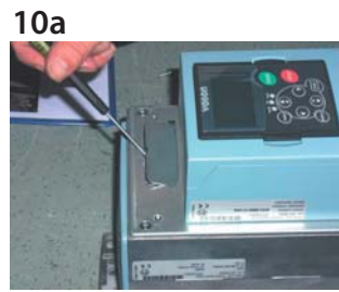
10a Remove the plastic cover of the frequency converter and open the small lid on the power unit cover. Leave the opening uncovered.
