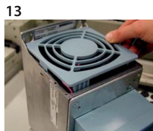
13 Carefully re-install the fan ensuring that the connector clip fits accurately. Do not slam, do not force!
