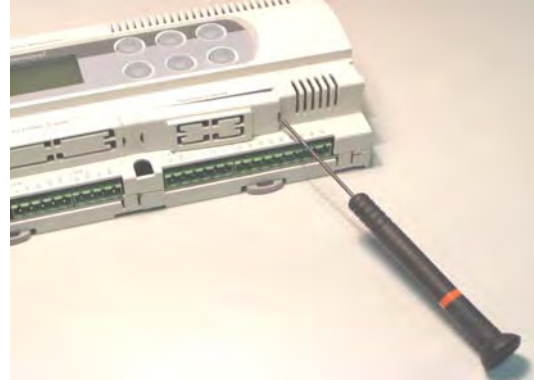
Figure 2.b – Removing the cover from the pCO controller
