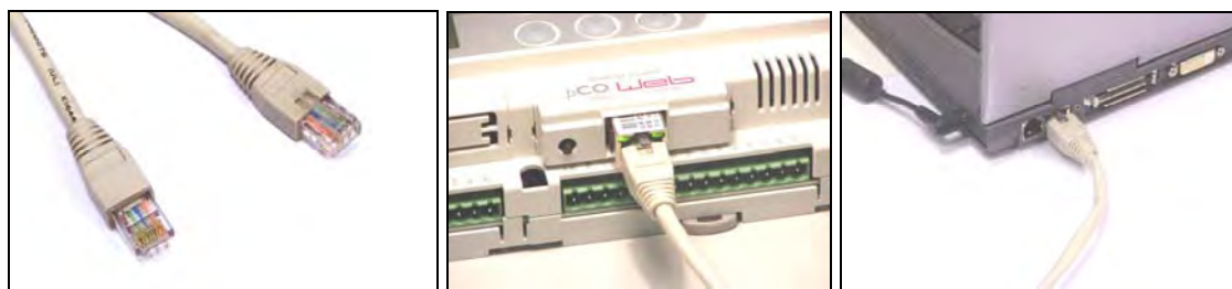
Figure 3.f – pCOWeb - PC connection
