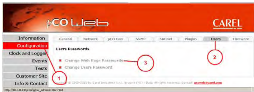
Figure 9.v – Protection and access control
