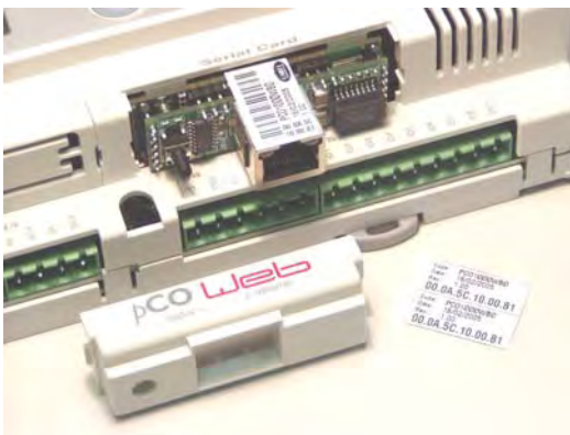
Figure 2.c – Inserting pCOWeb in the pCO controller
