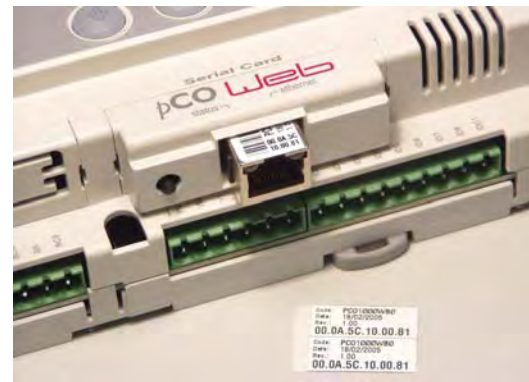
Figure 2.d – Securing pCOWeb with the cover
