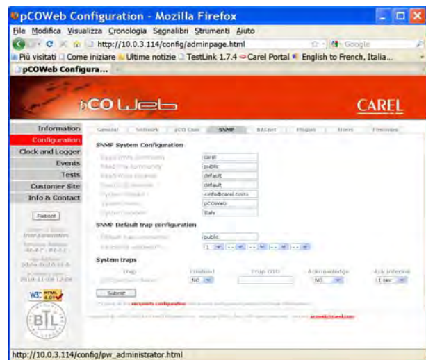
Figure 6.b - SNMP: basic configurations
