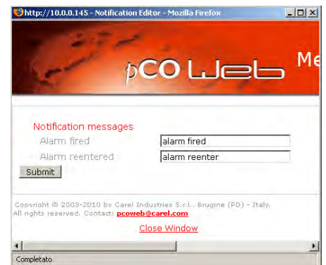
Figure 4.r – Setting the strings sent for Activation - Return
