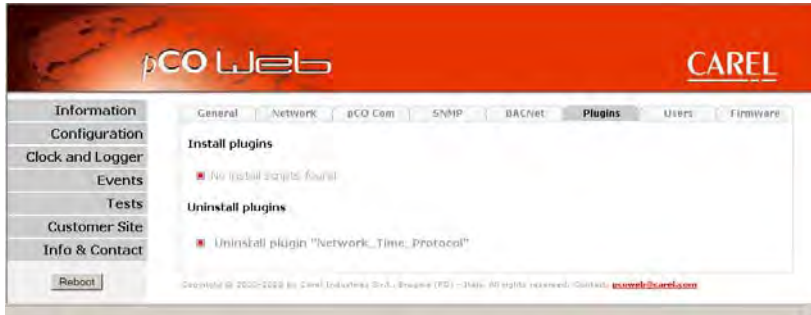
Figure 9.t – Install/Uninstall Plugin page after having installed “NTP”
