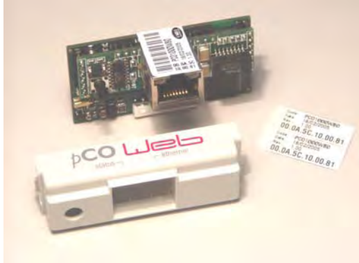
Figure 2.a – pCOWeb and the accessories supplied
