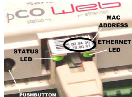
Figure 1.b - MAC address and indicator LEDs
