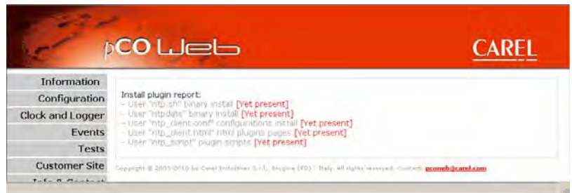
Figure 9.q – “NTP” Plugin installation report if the Plugin is already installed
